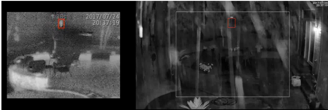
SightSensor (at left) detects the intruder accurately at night in heavy rain (at right).
