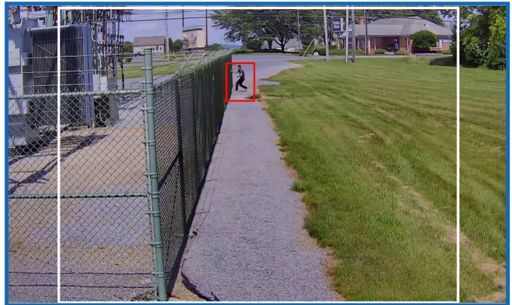
White border indicates thermal detection zone
